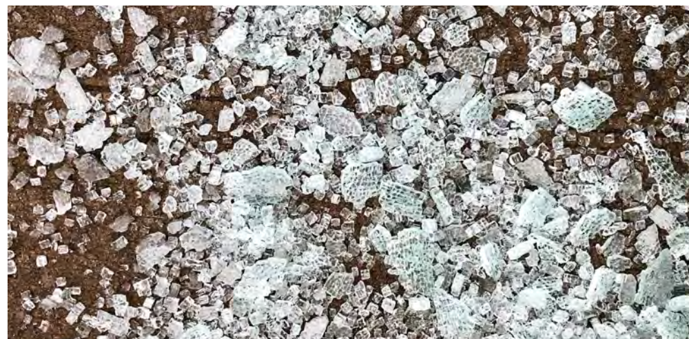
Shopfront with broken toughened glass
