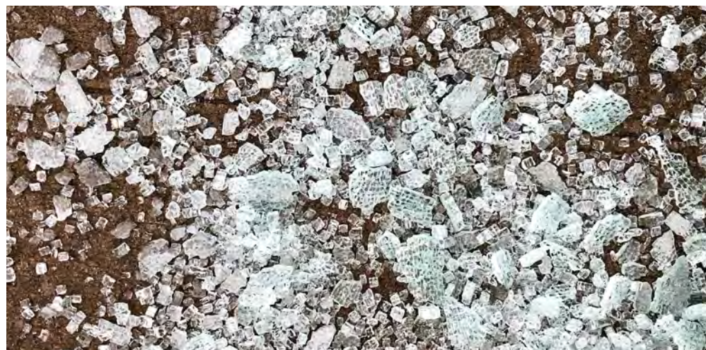
Shopfront with broken toughened glass
